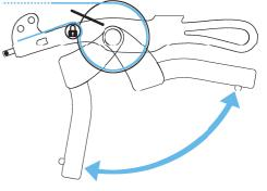
11.3 Remove the lock (9) by pulling the bow.
